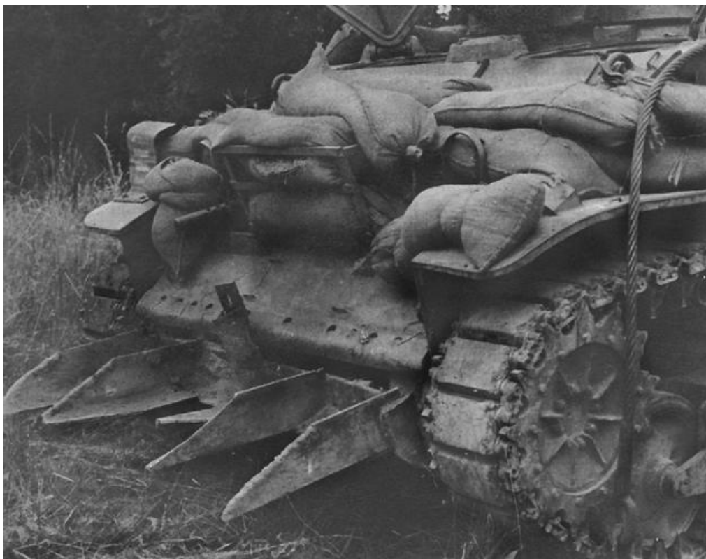
Tank with Hedgerow Cutter and Sandbags U.S. Army Center for Military History
